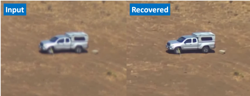
Figure 1.6: A monitoring application of techniques developed for imaging through turbulence. Shown in this figure is a reconstruction result for an airborne image.
