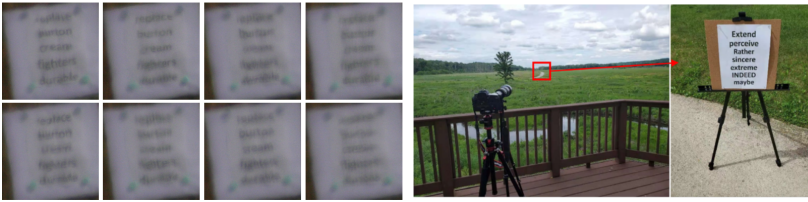
Figure 5.18: Real text data collected by an off-the-shelf camera with an optical zoom. Shown on the left are example distorted images, whereas the subfigures on the right are the actual camera setup.
